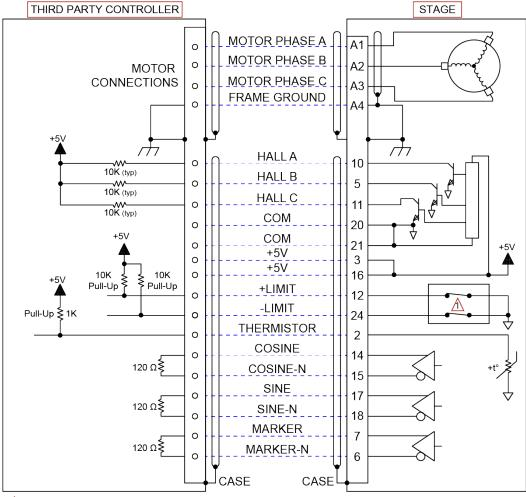
Figure 3-2: ANT130L Motor and Feedback Wiring [-CN2 Option]
