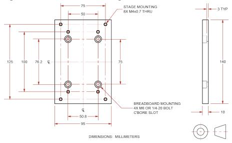
Figure 2-5: **ANT95L-075 Dimensions** STAGE CABLE MIN LENGTH 750
