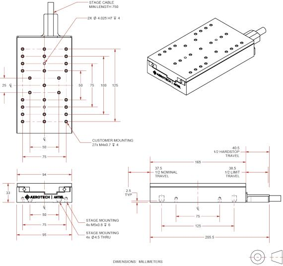
Figure 2-6: **ANT95L-075 Mounting Plate Dimensions**
