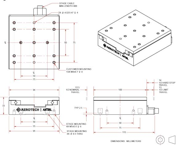
Figure 2-2: ANT95L-025 Mounting Plate Dimensions
