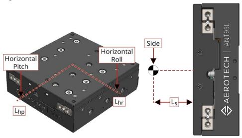
Figure 2-11: Cantilevered Load Capabilities
