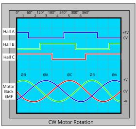
During CW rotation, each Hall effect signal is at a logic high state when its corresponding motor phase is at a negative voltage.
