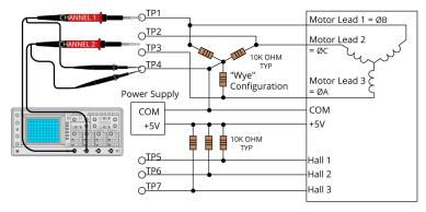
After the phase relationships of the motor have been determined, the next step is to determine the phase relationships of the Hall signals. The expected relationship between motor BEMF and the Hall signal is the peak of the BEMF. This relationship should correspond to the low voltage phase of the Hall signal. The relationship is shown in Figure 2-6.
