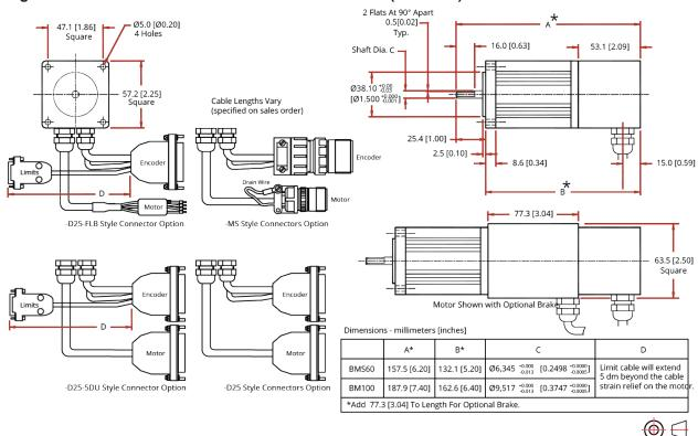
Figure 1-11: BMS60 and BMS100 Model Dimensions (NEMA 23)
