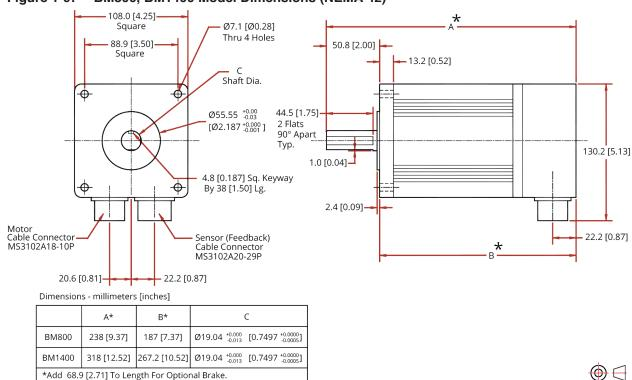
Figure 1-9: BM800, BM1400 Model Dimensions (NEMA 42)
