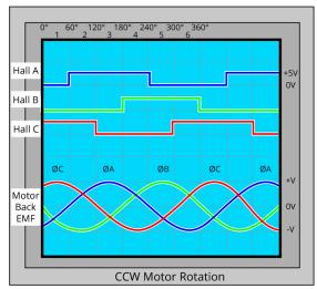
During CCW motor rotation, each Hall effect signal is at a logic low state when its corresponding motor phase is at a negative voltage.
