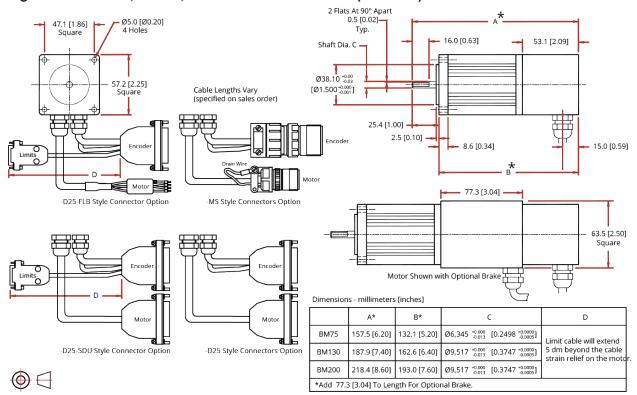
Figure 1-7: BM75, BM130, BM200 Model Dimensions (NEMA 23)
