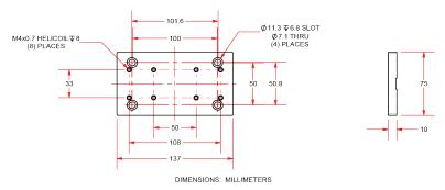
Figure 2-3: MPS75SL/SLE-025 Mounting Plate Dimensions
