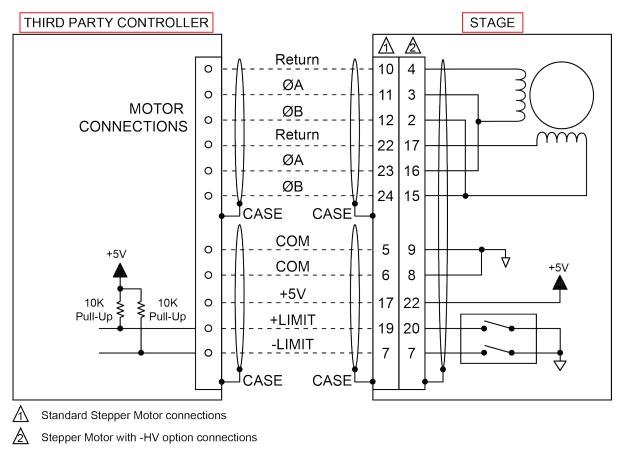
Figure 3-2: Motor and Feedback Wiring (-M2 Option)
