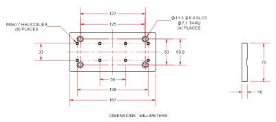
Figure 2-4: MPS75SL/SLE-050 Mounting Plate Dimensions
