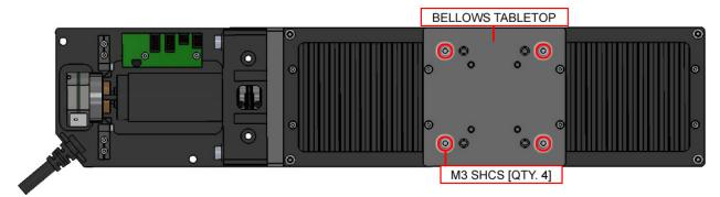
Figure 4-8: Attach the Bellows Tabletop
