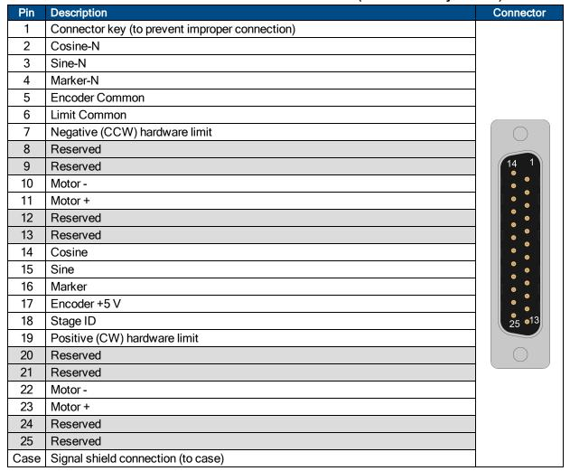
Table 3-2: 25-Pin D Motor Mating Connector (-M1)
