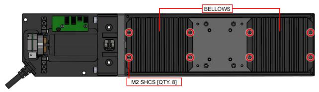
Figure 4-6: Attach the Bellows
