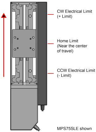
Figure 3-3: Machine Direction
