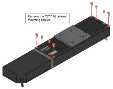
Figure 4-1: Remove the Bellows Bolts
