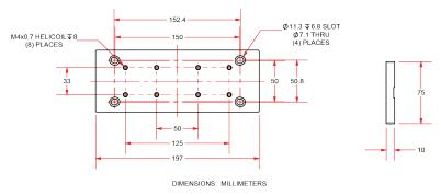
Figure 2-5: MPS75SL/SLE-075 Mounting Plate Dimensions
