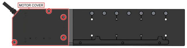
Figure 4-3: Motor Cover Screw Location
