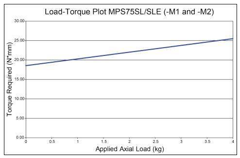
Figure 2-12: Torque Required to Turn Ball Screw in Vertical Orientation
