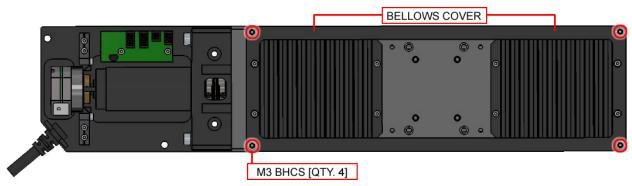
Figure 4-7: Attach the Bellows Cover
