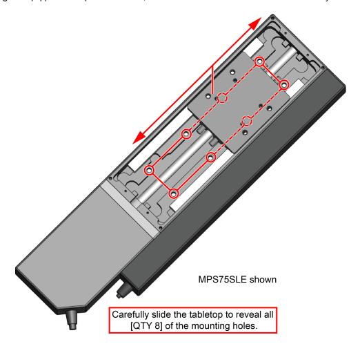
Figure 2-9: **Access To All Mounting Holes**
