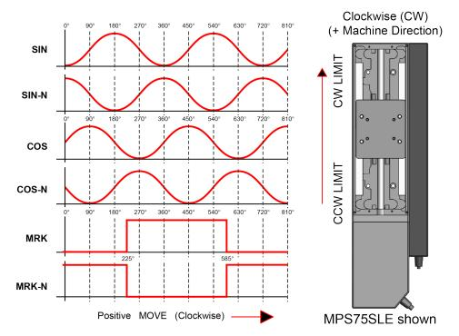
Figure 3-4: Analog Encoder Phasing Reference Diagram
