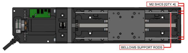
Figure 4-5: Secure the Bellows Support Rods
