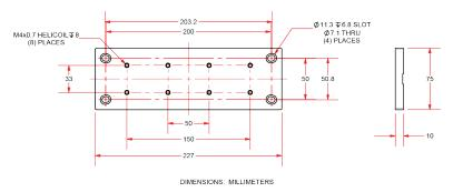
Figure 2-6: MPS75SL/SLE-100 Mounting Plate Dimensions
