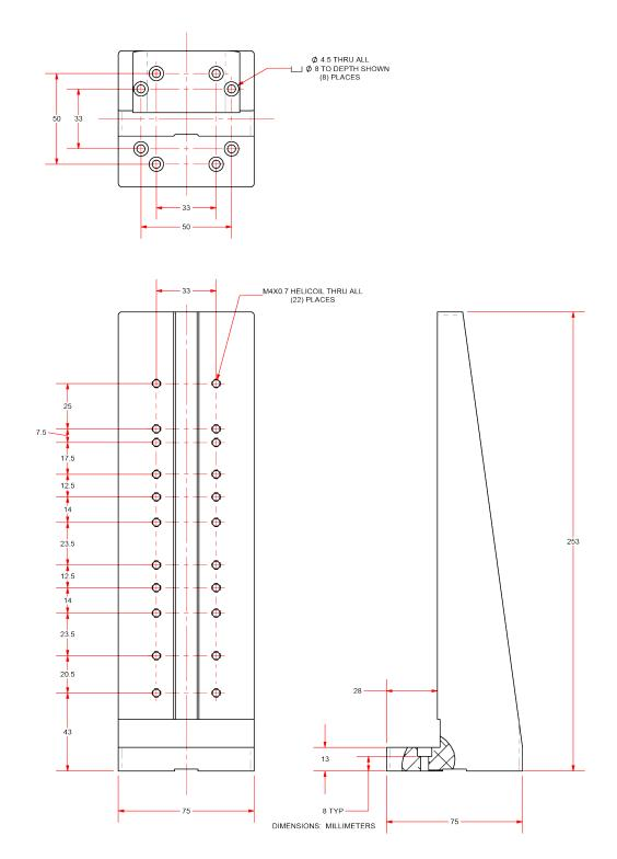
Figure 2-7: MPS75SL/SLE HDZ Angle Bracket Dimensions
