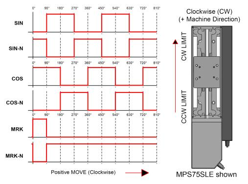
Figure 3-5: Encoder Phasing Reference Diagram (Standard)
