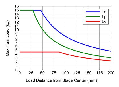
Figure 2-10: Load Capability of MPS75SL/SLE Series Stages
