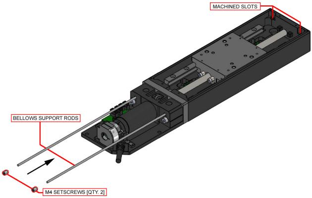
Figure 4-4: Bellows Support Rods
