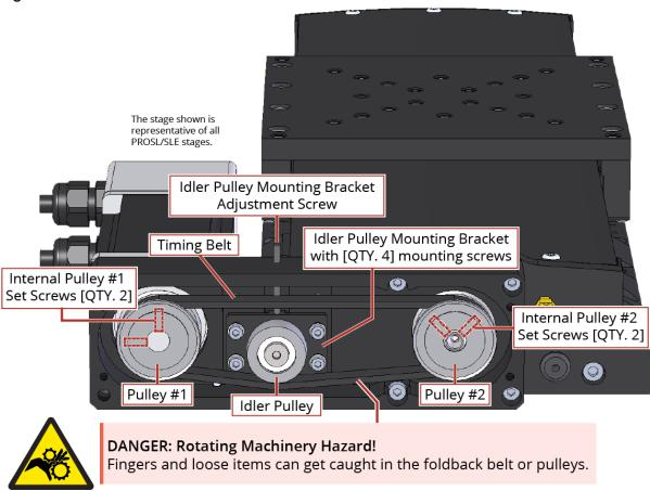
Figure 4-18: Lubricate the Pulley Flanges
