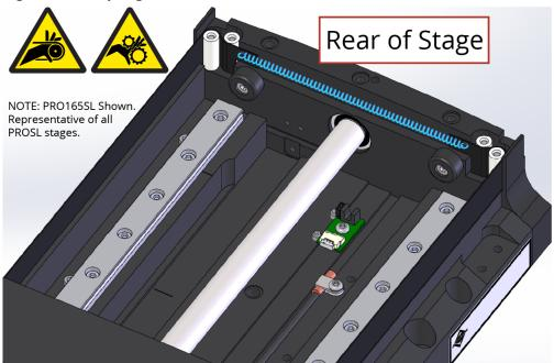
There are two methods that you can use to install the new belt through the stage table: **Pull Through Method**: Use this method if the old belt is intact and fed through the stage table. **Manual Feed Method**: Use this method if the old belt is not fed through the stage table.
