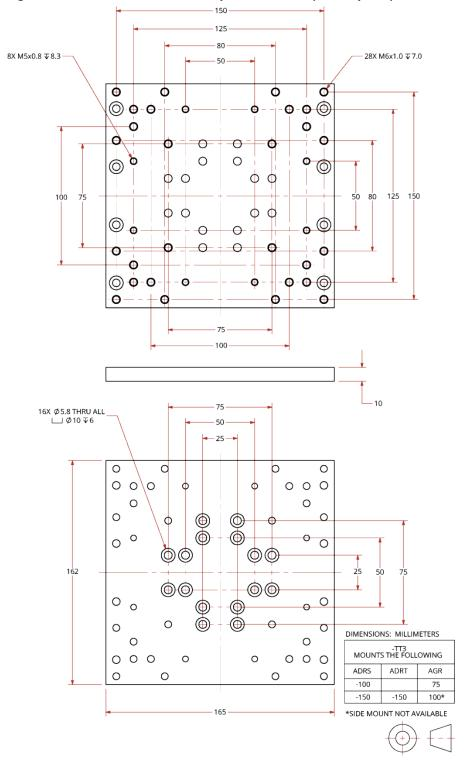
Figure 2-4: PRO165SLE Tabletop Dimensions (-TT3 Option)
