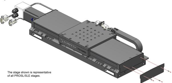
Figure 4-2: Hardcover Screw Removal
